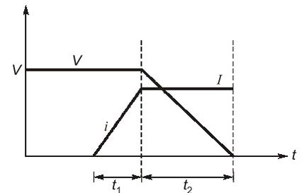
**Q2** Find the energy loss during switch-on and off intervals of a power transistor with switching characteristics as shown in the figure. Where  $I_{CS} = 80$  A,  $V_{CC} = 220$  V,  $t_{on} = 1.5$  ms and  $t_{off} = 4$  ms. Also determine the average power loss in the transistor if switching frequency is 2 kHz.
